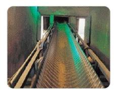
Chevron conveyor belts are highly effective for transporting sand, coal powder, grain or other powder or granular materials or materials packed in bags or boxes on incline though they can transport coal or mineral ore just like ordinary conveyor belts. They can transport powder or granular materials on 17°~28° inclines and materials packed in bags or boxes on 30°~35° inclines.
